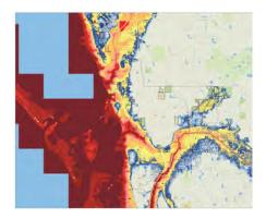
Using Geographic Information System ArcMap software, we geo-spatially mapped infrastructure and organized it into an interactive database. The maps helped visualize the infrastructure grid and provided a foundation upon which to model climate hazards. Light Detection and Ranging (also known as LiDAR) and digital elevation model tools were used to estimate ground elevations to better understand localized conditions surrounding infrastructure assets.
