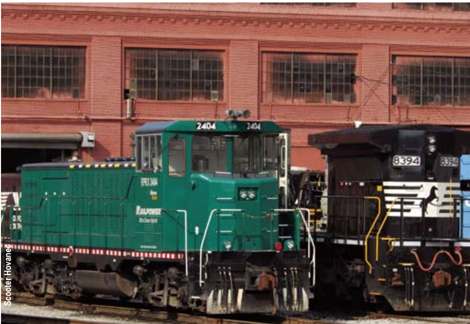
Hybrid locomotives, such as RailPower's Green Goat, use batteries instead of generators to power traction motors. A small diesel engine keeps the batteries charged.
