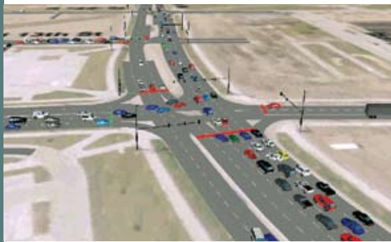
Computer simulations used event data to show effects the new stadium would have on traffic operations.
