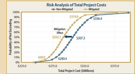
Risk assessment findings: The figure shows the probability distributions of construction costs of mitigated versus non-mitigated scenarios. The graphic depicts potential savings that can be realized if mitigation measures take place.
