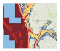
Using Geographic Information System ArcMap software, we geo-spatially mapped infrastructure and organized it into an interactive database. The maps helped visualize the infrastructure grid and provided a foundation upon which to model climate hazards. Light Detection and Ranging (also known as LiDAR) and digital elevation model tools were used to estimate ground elevations to better understand localized conditions surrounding infrastructure assets.
