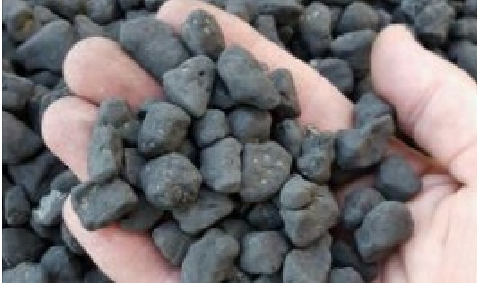
Figure 6-8. Inorganic biofilter media, Biorem Biosorbents
