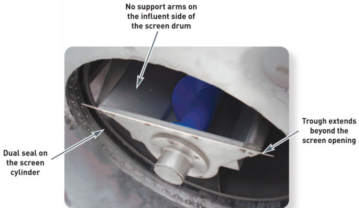
Figure 3-6. VFA1200-DM SAVI BEAST screen features
