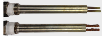
Figure 2. Examples of LPR Probes with Corroded Electrodes
